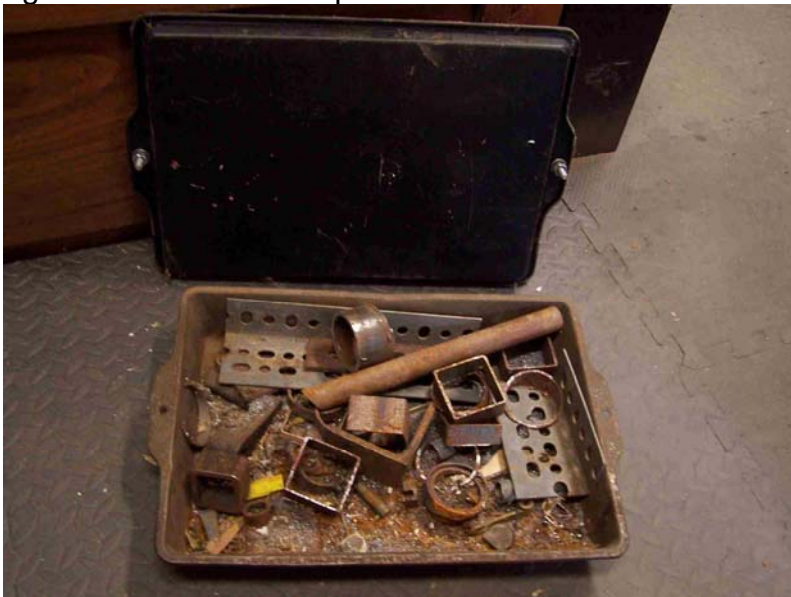
Chip tray is two garage sale baking pans sitting on angle irons attached to saw legs. Note two protruding 5/16 bolts that position the lower pan to the angle irons and enable quick removal for C-clamp use.
