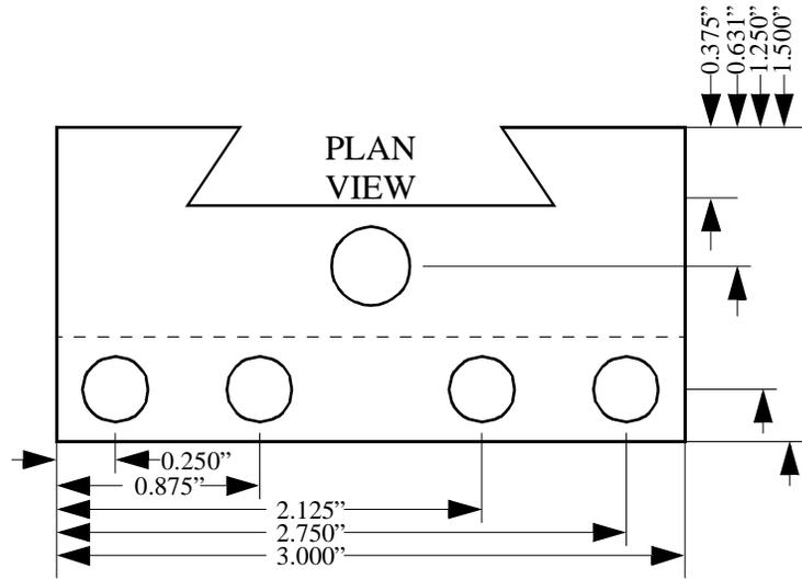
NOTE: Cut dovetail to match an existing Aloris toolholder.
