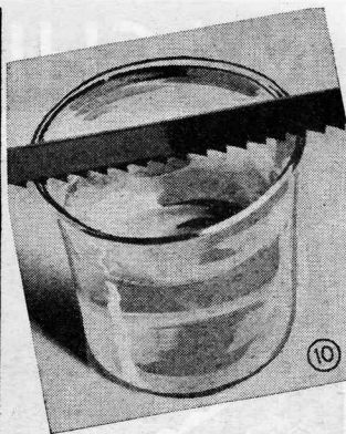
8—Teeth are milled in as many as forty saw bands at once, the bands being clamped side by side in an air-operated vise. 10—Acid test shows exact depth of flame-hardening on saw bands by discoloring hardened portions. 9—Tooth-setting machine that shows a magnified image of the teeth between limit lines so that operator can detect errors of set at a glance. The circular insert shows image as seen
