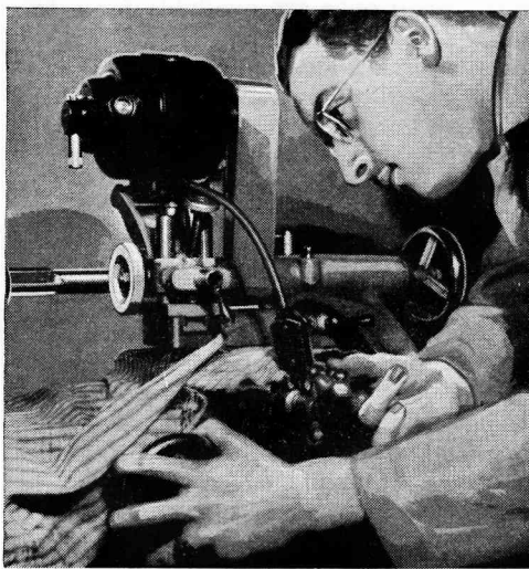
⑰ FINISH-GRINDING THE SHANK
