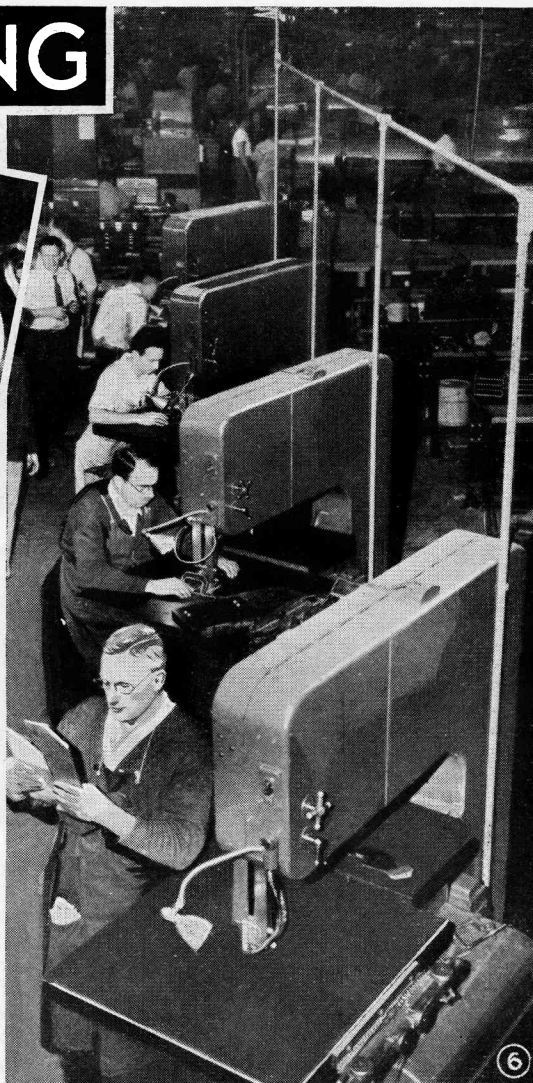
6—Batteries of contour machines are found in many large production plants, forty or fifty units not being unusual. 7—Metal for saw bands being tested for grain structure with a metalscope, which shows enlarged views and makes photomicrographs
