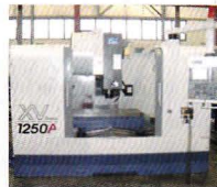
SUPERMAX Vertical Machining Center, Model: XV-1250A (New 2001) GM#1775
