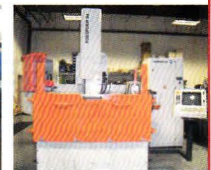
CHARMILLES Sinker-Type CNC EDM Machine, Model: Roboform 84, S/N 720.027, (New 2011) GM#1857
